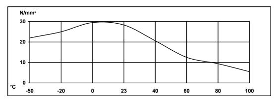
Roller peel test (ISO 4578) at 23°C Glass transition temperature (Tg) Tensile strength ISO R527 type 1 Elongation at break ISO R527 type 1: Coefficient of thermal expansion (-30°C/+30°C) 8.1 N/mm (cured 7 days at 23°C) 54°C (cured 7 days at 23°C) 25 MPa (cured 7 days at 23°C) 2.3 %
