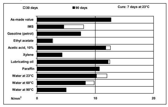
Lap shear strength versus tropical weathering (40/92, DIN 50015; typical average values)
