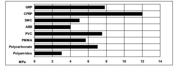
Cured for 16 hours at 40°C and tested at 23°C. Pretreatment - Lightly abrade and alcohol degrease.
