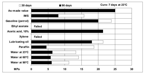
Lap shear strength versus immersion in various media at 23°C (typical average values). Substrate – aluminium
