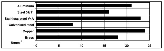
Average lap shear strengths of typical non-metallic joints (ISO 4587)
