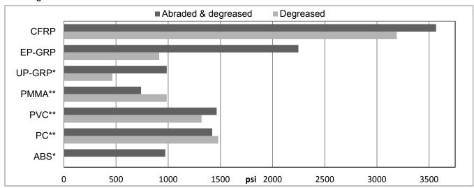
(\*): UP-GRP, ABS, substrate failure observed when abraded and degreased.
