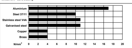
Cured for 24 hours at 23°C + 1 hour at 130°C and tested at 23°C Pretreatment - Sand blasting
