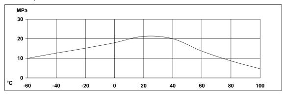
Roller peel test (ISO 4578)
