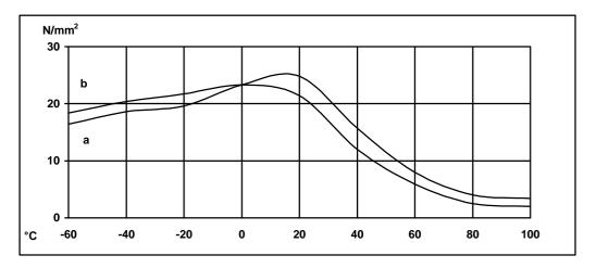
Roller peel test (ISO 4578)
