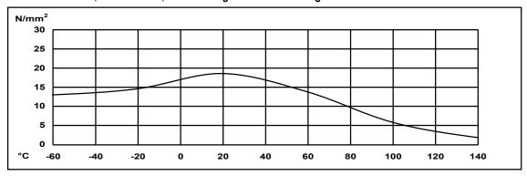
Other typical characteristics Cure: 72 hour/25°C, tested at 25°C, Sand blasting steel-Sand blasting steel
