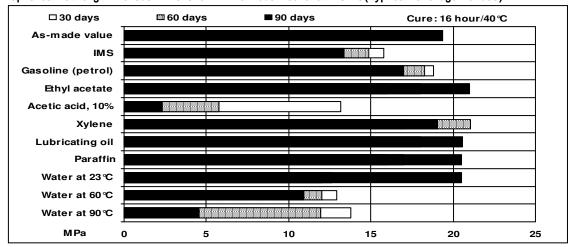
Lap shear strength versus tropical weathering(40/92,DN 50015)
