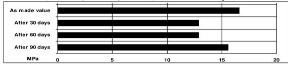
Lap shear strength versus heat ageing (ISO 4587)
