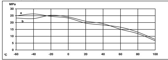
Tensile properties (ISO 527). Cure 16hrs at 40 °C (typical average values)- tested at 23 °C
