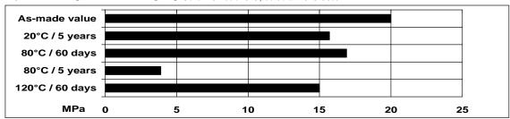
Lap shear strength versus tropical weathering Cure: 16 hour/40°C, tested at 23°C
