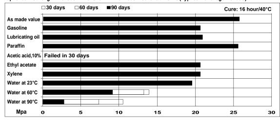
Lap shear strength versus heat ageing Cure: 16 hour/40°C,tested at 23°C 50% rh
